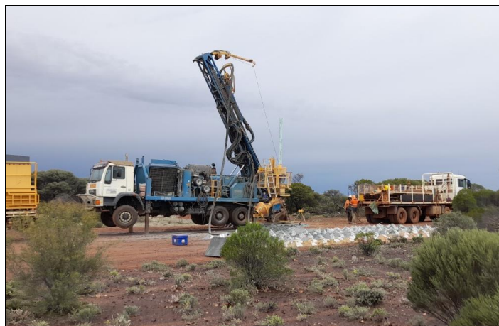
Figure 2 – Watsons Well RC Drilling.
