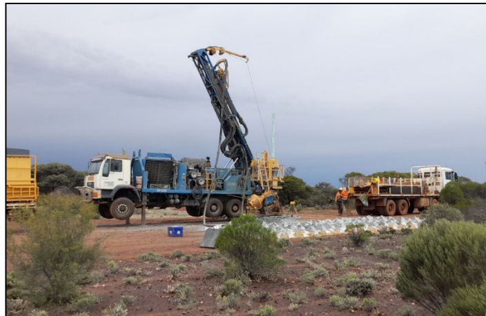
Figure 2 – Watsons Well RC Drilling.
